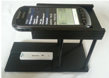
Figure 2: A plastic stand holds the mobile device in a convenient position above the RDT.
